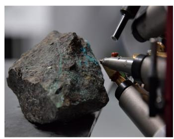
*Fig. 3 PIXE analysis of a chrysocolla veinlet,* © *S. Manya, C2RMF*
