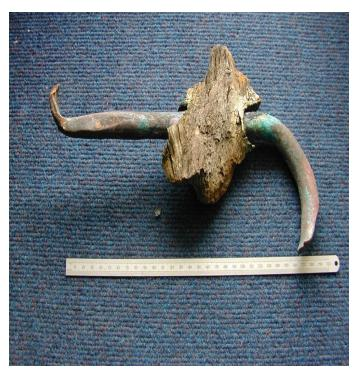
Fig. 2 Copper bolt from HMS Pomone
