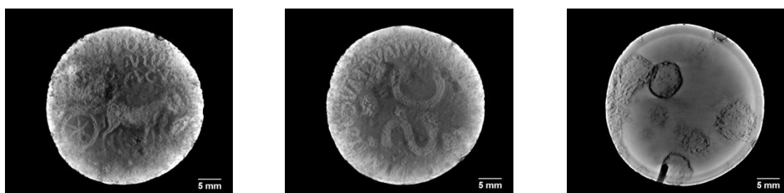
Figure 1 a-c: 3D- \mu CT imaging a sestertius of Tiberius obverse (a), reverse (b) and inner part of the coin (c) with drill hole and showing depletion of zinc
