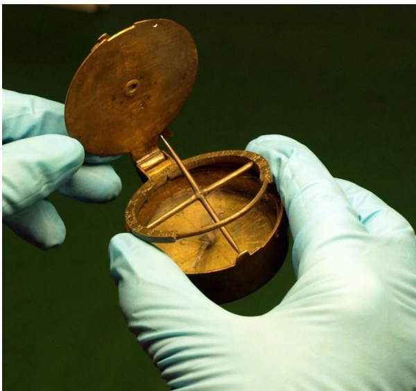
A compendium, c. 1450, made from copper-alloy and comprising a magnetic compass, an equatorial sundial and a simple nocturnal, now in the Oxford Museum of the History of Science. (Photo: J Davis)
