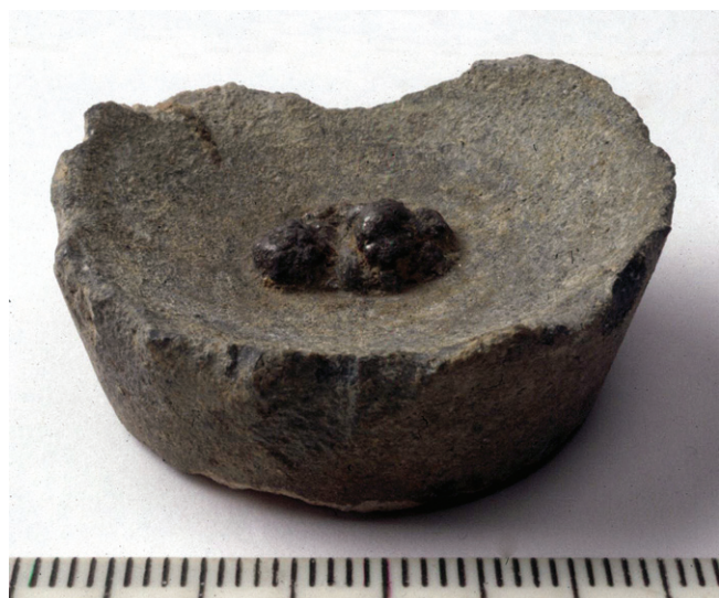
Figure 76: A bone ash cupel from Cripplegate, London, with the silver that was assayed in it still in position. Scale in mm.
