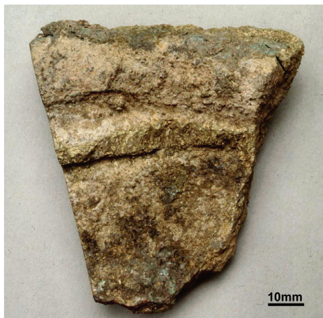
Figure 75: Fragment of the lining of a 13th-century cupellation hearth impregnated with lead oxide (also known as a litharge cake) from Thetford, Norfolk.
