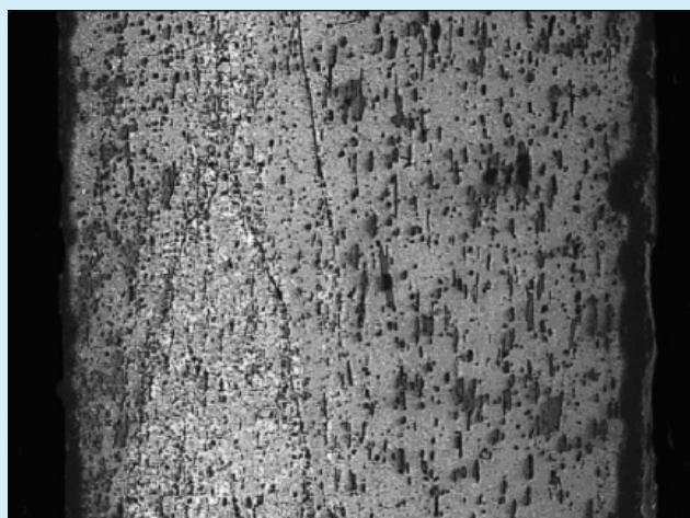
Figure 22: Section through knife blade. The varied texture to the left shows the incorporation of several pieces of scrap metal. Image width ~1.5mm.
