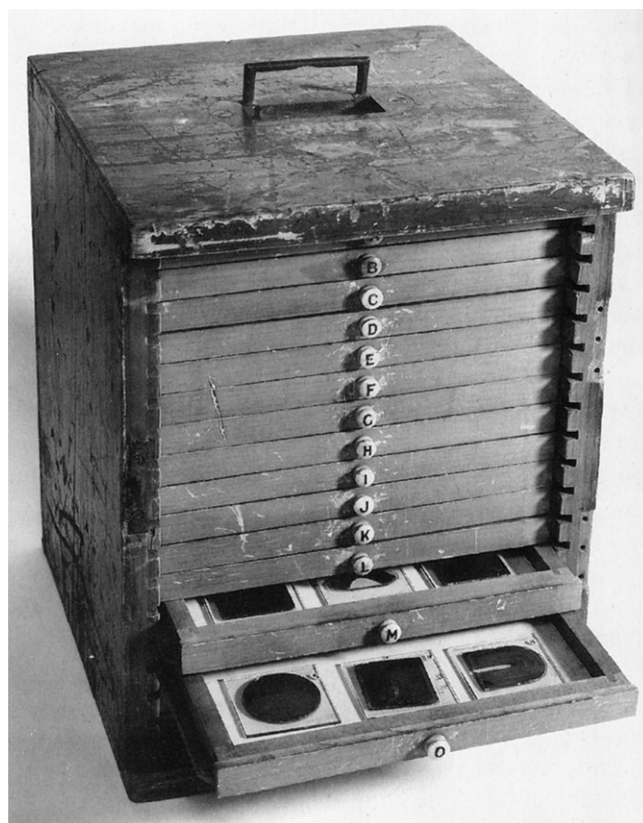
Figure 29: Cabinet containing polished metallurgical samples made between 1863 and 1865 by Henry Clifton Sorby, the pioneer Sheffield metallographer. Now in the collections of the South Yorkshire Industrial History Society.
