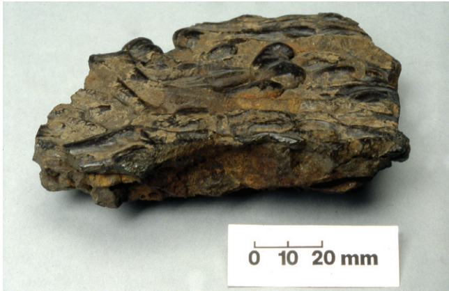
Figure 16: Tap slag, showing its characteristic flow-form surface structure.
